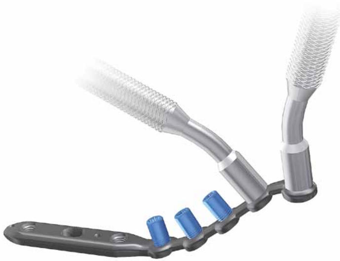
Figure 9 The plates can be contoured up to 45 degrees at each bridge between the F.A.S.T. Guide inserts.
