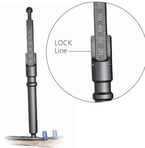
Figure 32 Take reading directly from the LOCK Line on the Small Fragment Depth Gauge.
